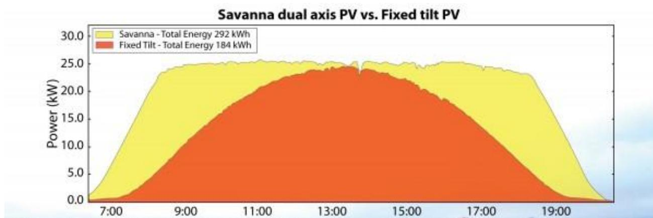
The main advantage of such systems is their complete autonomy. This advantage is in line with the main, because in the work of dynamic systems do not need the human power cost, in general intervention without the need will bring only losses. The mobile system autonomy is a positive and effective advantage over the static system of the solar power plant.
