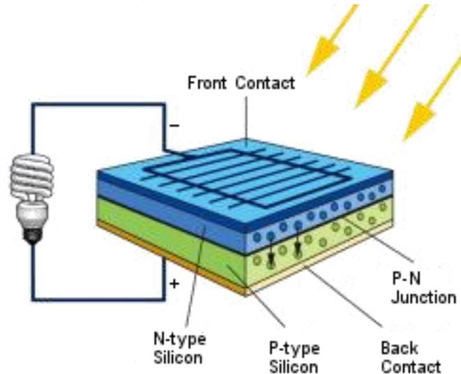
Figure 1 - Scheme of work of solar panels
