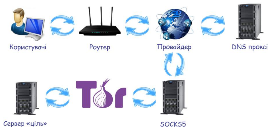
Figure1 – scheme of the multi-level data protection algorithm
